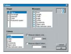
Ellix automatically recognises objects by elliptic, circular, rectangular approximation in order to determine their length, width, surface, orientation and shape factors.
