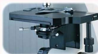
Smooth, coaxial control mechanical stage with slide holder
