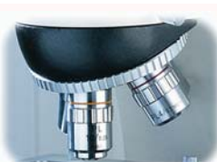
Reversed nosepiece with plan achromatic objectives
